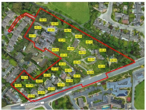
Figure 8-1 – Topographical Survey Extract
